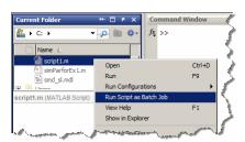
Running a script as a batch from the browser uses only one worker from the cluster. So even if the script contains a parfor loop or spmd block, it does not open an additional pool of workers on the cluster. These code blocks execute on the single worker used for the batch job. If your batch script requires opening an additional pool of workers, you can run it from the command line, as described in "Run a Batch Parallel Loop" on page 1-9.
